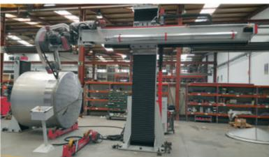
Machines for internal and external belt grinding and polishing of bottoms/dishes and tank bodies for food, pharmaceutical, liquid transport and chemical industries, etc.
