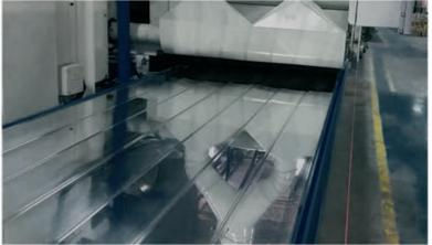
**Polishing machines for aluminum profiles** and flat parts with 1 or 2 working tables of 1000x7000mm.
