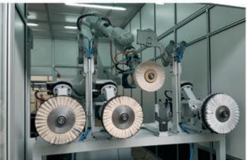
**8-axis robotic cell** with automatic loading of up to 4 tools for car window trim polishing. Piece holding table with capacity for 2 parts allowing loading and unloading during the working cycle.
