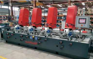
"Centerless" type belt grinding and polishing machine with universal heads for finishing tubes and round bars with diameters from 6 to 150mm.
