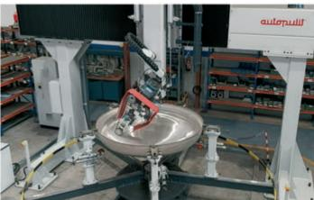
**Specific CNC machine** for belt grinding, polishing and satin finishing of bottoms/dishes up to Ø6000mm, both inside and outside, for food, pharmaceutical, liquid transport and chemical industries, etc
