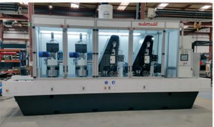
**Belt grinding and deburring machine** for fine blanking and stamping parts for the automotive sector, including of 2 belt grinding heads, 2 planetary heads with brushes and magnetic conveyor table for the correct fixing of the parts.
