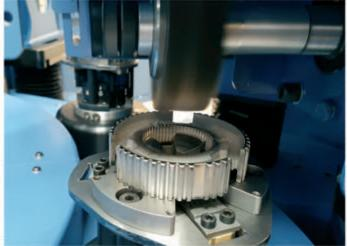
**High production capacity rotary transfer machine** for deburring sintered gears for the automotive sector.
