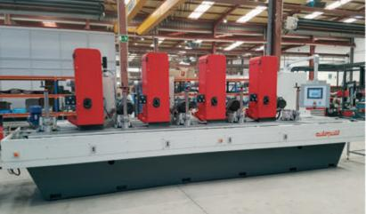
**Belt grinding and polishing machine** with universal heads for finishing square tubes, plates and flat parts.
