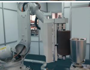
**7-axis robot cell** with automatic change of up to 5 tools for weld dressing and satin finishing of stainless-steel worktops, vats, dishwashers, sinks, etc., for the HORECA sector. Piece holding table with capacity for 2 parts allowing loading and unloading during the working cycle.
