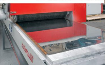
**Polishing machine for sheet metal** and flat parts. Table of 1250×3000 mm with alternative movement and polishing head with oscillation and automatic installation of polishing compound.
